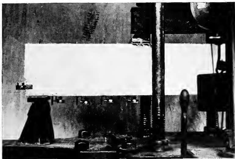
(b) Showing Instruments for Measuring Slip of Bar at End and at Intermediate Points.
